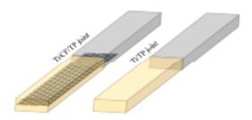
**Fig. 2:** Schematic diagram of joining samples with and without carbon fiber.
