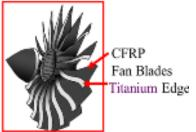
**Fig. 1:** Application of carbon fiber reinforced polymer (CFRP) with Ti sheath recently utilized for fan blades of turbo fan engines of airplane.
