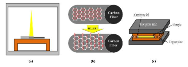
**Fig. 3:** Schematic drawing of joining process for carbon fibers wrapped by molten Ti (a), carbon fibers treated by *HLEBI* (b) and carbon fibers wrapped by melted polymer (c).
