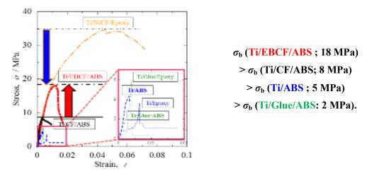
Fig. 4: Tensile stress-strain curves of Ti/EBCF/ABS and Ti/CF/ABS, together with Ti/ABS joints with and without glue.
